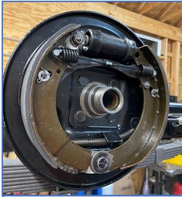
The MGTC's typical brake drum. This one is the rear right. If you look closely you can see the spring wound emergency brake cable.
