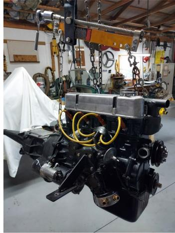
Rebuilt engine hanging and going back in for the first time. Not the last since frame/chassis modifications are needed.
