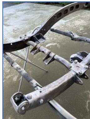
*The MGTC's frame showing its bare metal.*
