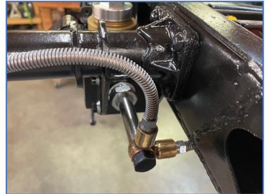
The MGTC's main brake pipe junction direct from the master cylinder routing fluid to front right wheel cylinder (bottom connection) then to another junction route.
