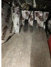
The floor mat padding needed to be shaped to fit the lowered floor of the car. Early E Types had flat floors but tall Americans didn't have enough leg room (The development driver, Norman Dewis, was impressively short and didn't notice the lack of legroom). Jaguar lowered the floor by inserting a dish like insert into it. BAS supplied a shaped floor mat and a pad that needed gluing along two shaped cuts in it to fit snugly.
