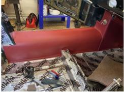
I began with the left side sill vinyl. The pieces (foam and vinyl) had been cut to shape by BAS and installing them was not too bad. A good place to get used to the way things would fit and stick down. Next came the Hardura side trim, which was pre-cut, bound and already had a hole in it for the bonnet latch handle. These two pieces gave me a bit of confidence that I would be able to handle the rest.
