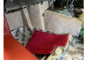
The other footwell sides had padding and carpet. Again, the pieces were already cut to shape and size. I glued the padding into place, then the carpet. It was interesting getting it to fit round the contours of the tunnel. This covered the bulkhead and gearbox tunnel on that side. After gluing the crossmember carpet in place the two floor mats just plopped into place.
