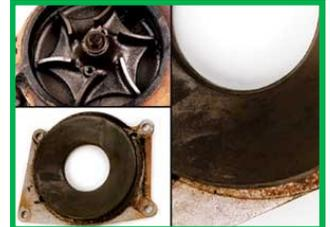
Original Water Pump from Caterpillar Engine with More Than 750,000 Miles Using Extended-Life Coolant (ELC).
