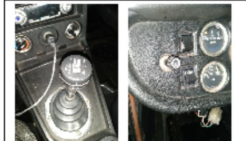
Overdrive switch should be on the gearlever knob. Now it's the upper rocker switch on the dash.
