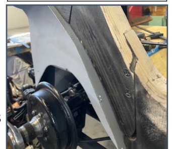
Rear right-hand side showing the wheel well lip. It should fit flush to
