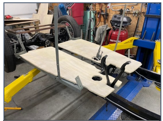
New floorboards cut from 1/2" plywood.
