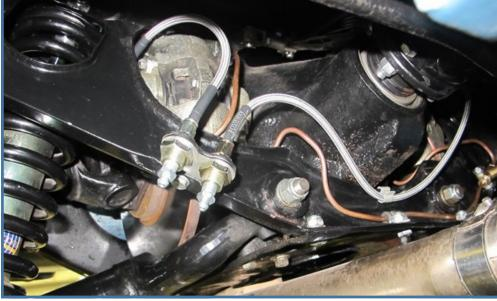
Dave Maule has been addressing brake problems on his Austin Healey 100 recently. After rebuilding his front calipers while he was reinstalling the lines, I noticed the fittings on the short lines that connect the
