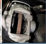
to rebuild them completely once again. On inspection, stainless pistons previously installed were great. All the rubber components were shot. It seemed the rubber boots welded the pads in place acting liked a rubberized glue.
