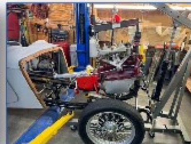
The MGTC EXU engine being lowered onto the MGTC chassis. Weight 1,850.
