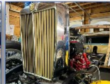
The unique MGTC chrome shell and grill mounted anticipating the installation of the engine cowlings
