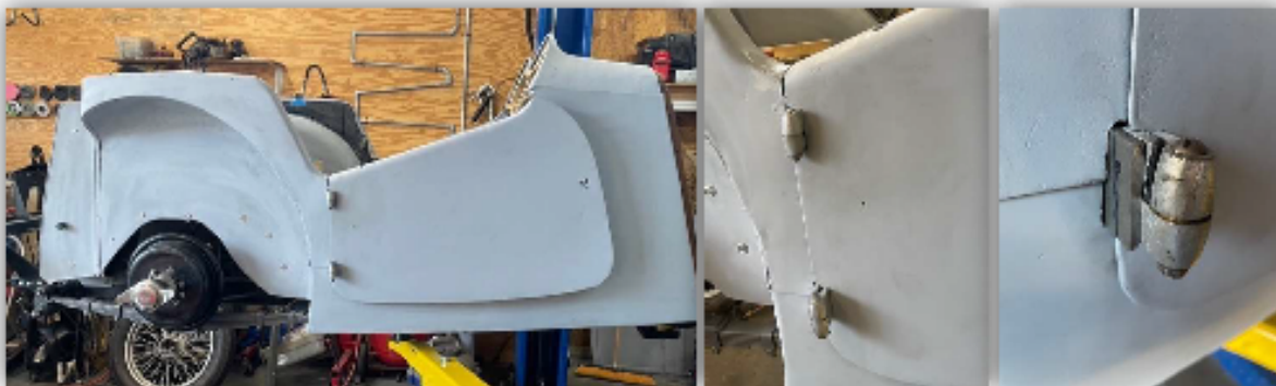
Driver's side door details showing the hinges and the preliminary shimming. Yes, some correcting is necessary!
