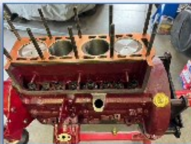
Top view showing the copper head gasket, 10 long head bolts and cam followers just visible in front.
