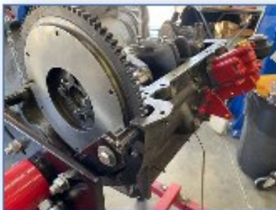
Bottom view showing the fly wheel and starter gear ring of the engine. Also, the oil pump in the back.
