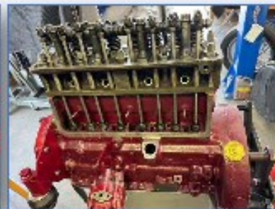
The installed head (not torqued). Also showing the CAM followers for exhaust and combustion.
