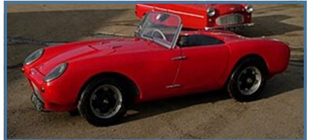
Power was provided by a 328cc Excelsior Talisman motor cycle engine producing all of 18 bhp. The 4 speed transmission was modified so that 1<sup>st</sup> gear was actually a reverse leaving the remaining gears as a 3 speed sequential box. Instead of the foot operated 1 up 3 down pedal shifter, gears were selected via single throw gated lever mounted on the floor, which operated in a manner similar to a modern automatic.
