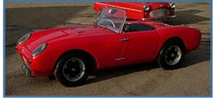
Power was provided by a 328cc Excelsior Talisman motor cycle engine producing all of 18 bhp. The 4 speed transmis-
