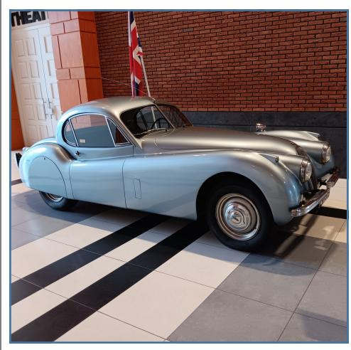
Powered by a 150hp 3.4 litre XK engine it was, at the time, the fastest production car in the world. The 120 in its name denotes its theoretical top speed of 120mph. A version driven by Jaguar test driver Norman Dewis actually achieved 220kph (nearly 137mph) in Jabbeke, Belgium.
