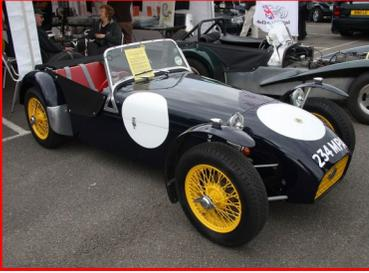
The Lotus Super Seven was introduced in 1957 as a replacement for the Mark VI. It was originally powered with a 36 horsepower Ford 1,172 cc side valve four cylinder engine (my second car was a Ford Prefect powered by the same engine). Since it was sold (in the UK) as a kit car many owners opted for something a bit more powerful and fitted the BMC A series or Coventry Climax engines. This car was more of a club racer than a road car.
