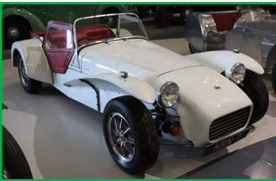
The rear axle (from a Standard Companion) was no longer up to the job and in the Series 3 (1969) was replaced by a Ford Cortina unit and generally had the crossflow engine. In 1969 the Lotus twin cam engine became available. It was the Series 3 that became the Caterham in the 70's.
