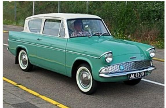
Three models were available - two door Saloon, three door Estate and two door panel van (which morphed into the Thames 307E van). Powered by the 997cc Kent engine, they topped out at 73.8 mph (yikes!) and shot to 60 mph in 26.9 seconds. All this for just £610 (about \$2457 in 1959) including taxes of £180.
