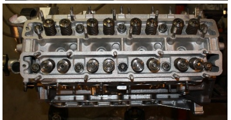
New Cylinder Liners, Pistons, Valves
